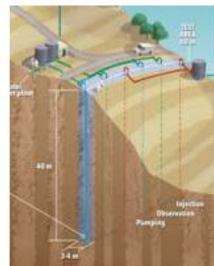
Implementation of infrastructures for the field test (accesses, boreholes, injection and pumping equipment, safety barrier equipment). Initial hydrogeological and tracer tests to establish the functioning of the aquifer and the conditions under which the definitive tests are expected to be conducted.
