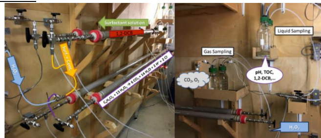
Figure 1: S-ISCO column test setup. Left: Flow scheme. Right: Sampling with gas traps and outflow bottles.
